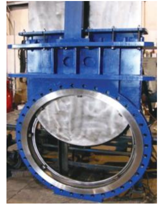
Left: 48" Figure 76 square bottom metal seated knife gate valve. Right: 42" Figure 76 round bottom metal seated knife gate valve.
