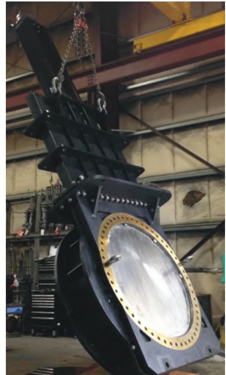
Figure 193 bonneted metal seat-ed knife gate valve with 60"x72" inlet and outlet, working in a Colorado dam.
